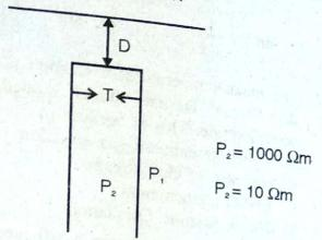
The dyke can be successfully mapped if the minimum skin depth and the transmitterreceiver distance are, respectively;
